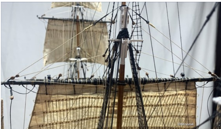
Close-up of the aft of the sail, where you can see the parrels and rigging.
